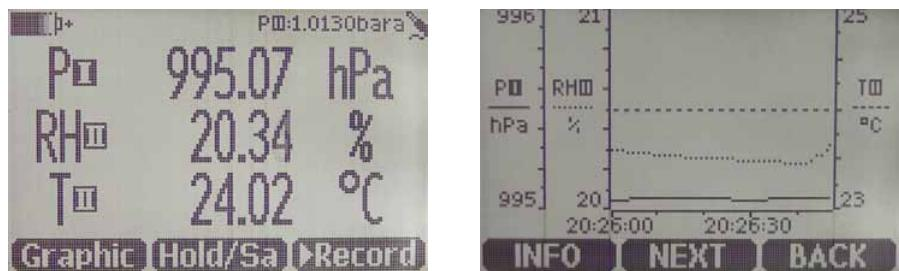
Some humidity measurement instruments allow an individual humidity parameter to be chosen which can then be followed on a graphical display. This picture shows different views of the Vaisala HUMICAP Hand-Held Humidity and Temperature Meter HM70 display.
